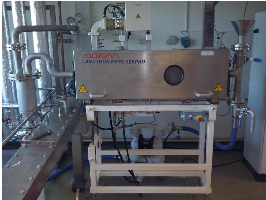
20 L scale MW rig (6 kW) able to withstand slurries, work in a semi-continuous up to 95°C and with a flow rate up to 200 L min<sup>-1</sup>
