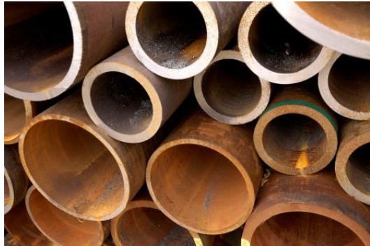
Rust develops on steel during transportation, handling and storage. → Material waste and higher costs
