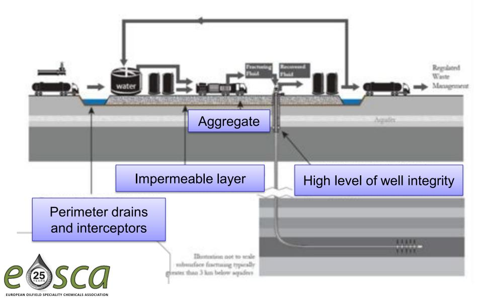
Transport of water, fracturing fluid products, and proppant from offsite
