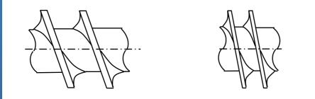
Large pitch Small pitch Conveying/ transport elements
