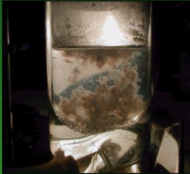
No ultrasound Amorphous-looking lumpy solid
