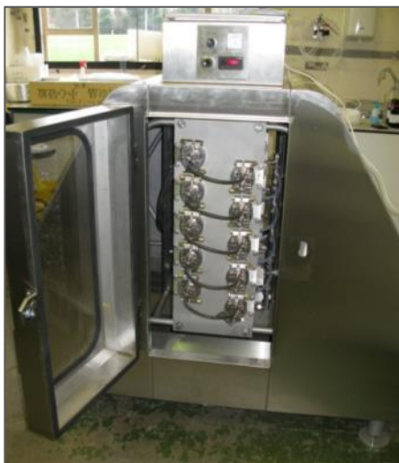
1-10 litre ATR flow reactor
