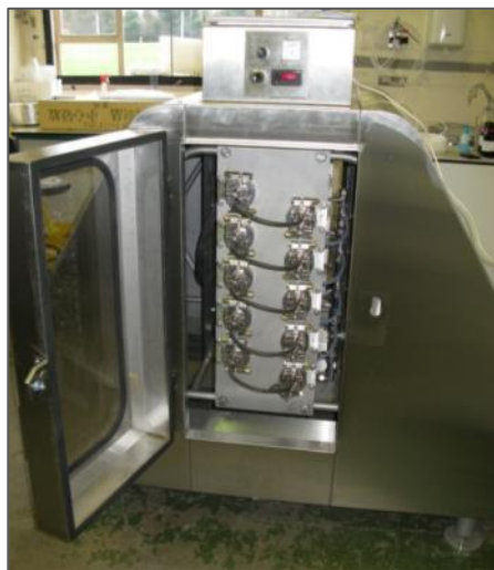
1-10 litre ATR flow reactor
